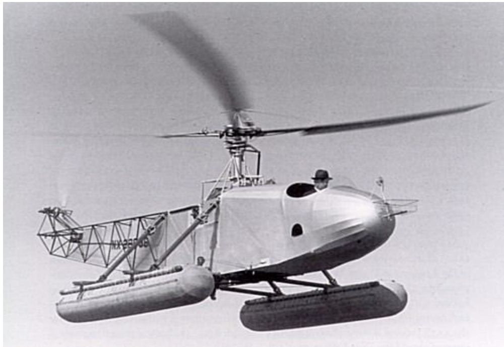
Figure 3.6 A VS-300 Piloted by Igor Sikorsky Towards the End of 1941 (source: http://en.wikipedia.org/wiki/Helicopter )
