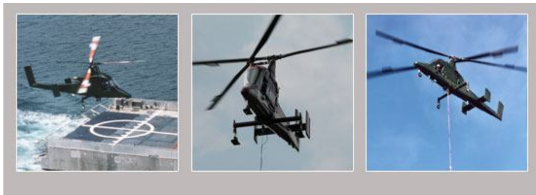
Figure 3.16: The K-Max Unmanned Helicopter is Based on the K-Max Heavy Lift Helicopter as Shown. (source: http://www.kamanaero.com/helicopters/uav.html )
