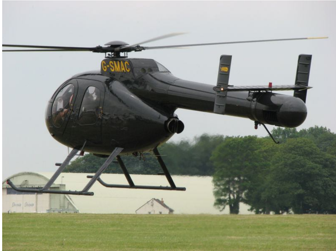
Figure 3.28: MD NOTAR Helicopter. (source: http://en.wikipedia.org/wiki/Helicopter )
