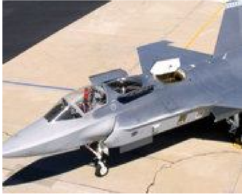
Figure B.3: X-35B Showing Lift Fan (source: http://upload.wikimedia.org/wikipedia/commons/thumb/7/78/F-13_lift_fan.jpg/180px-F-13_lift_fan.jpg )
