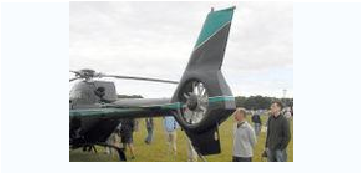
Figure 3.26: The Fenestron Tail System (source: http://en.wikipedia.org/wiki/Helicopter )
